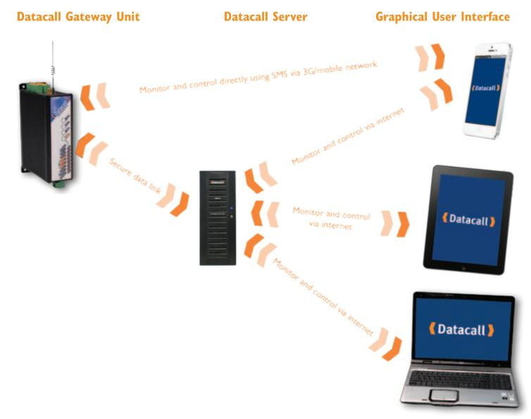
The **Datacall Telemetry System** offers a cost effective means to monitor and control remote assets using mobile networks and the internet. This powerful and flexible product is easy to set up and simple to use.
